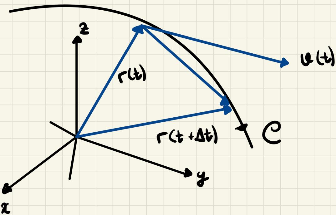
This velocity vector has direction tangent to the path  $C$  at the point  $r(t)$  and it points in the direction of motion. The length of velocity
