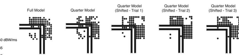
**IN THIS WORK, WE DESIGN OPTICAL COUPLERS FOR MAXIMUM POWER TRANSFER THROUGH BENDED NANOWIRE TRANSMISSION LINES. SPHERICAL PARTICLES ARE USED AT THE BEND LOCATIONS TO IMPROVE THE TRANSMISSION CAPABILITIES, EVEN FOR DIFFICULT SHARP BENDS. OPTIMIZATIONS ARE CARRIED OUT TO FIND THE MOST SUITABLE ARRAY STRUCTURES TO MAXIMIZE THE OUTPUT.**
