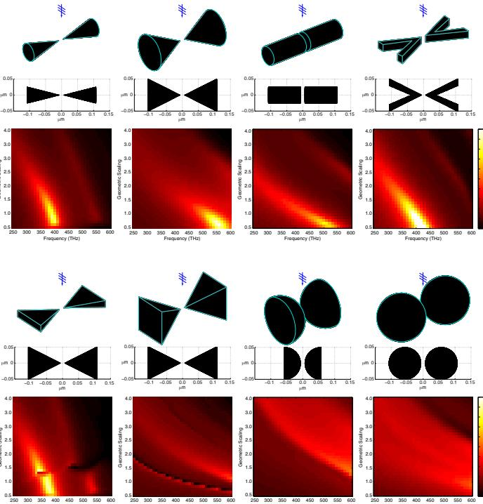
IN THIS WORK, WE STUDY DIFFERENT NANOANTENNA GEOMETRIES FOR POWER ENHANCEMENT (ENERGY HARVESTING) APPLICATIONS. SINCE ELECTROMAGNETIC SCALING IS NOT VALID FOR METALS AT OPTICAL FREQUENCIES, 2D INVESTIGATION IS REQUIRED FOR A FULL ASSESSMENT OF A GIVEN GEOMETRY. WE FIND CANDIDATE STRUCTURES FOR ENERGY HARVESTING AT DIFFERENT RANGES OF THE ELECTROMAGNETIC SPECTRUM. MULTIBAND OPERATION IS ALSO POSSIBLE FOR GEOMETRIES WITH SLITS.
