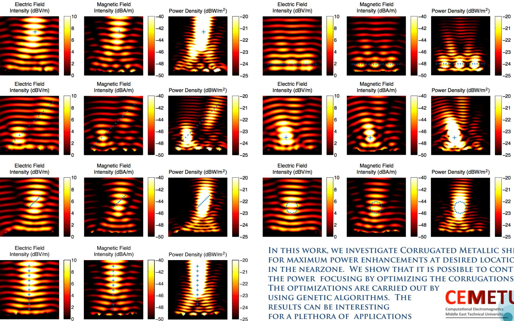
IN THIS WORK, WE INVESTIGATE CORRUGATED METALLIC SHEETS FOR MAXIMUM POWER ENHANCEMENTS AT DESIRED LOCATIONS IN THE NEARZONE. WE SHOW THAT IT IS POSSIBLE TO CONTROL THE POWER FOCUSING BY OPTIMIZING THE CORRUGATIONS. THE OPTIMIZATIONS ARE CARRIED OUT BY USING GENETIC ALGORITHMS. THE RESULTS CAN BE INTERESTING FOR A PLETHORA OF APPLICATIONS INCLUDING OPTICAL IMAGING.
