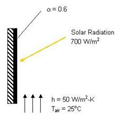
surface, as shown in the figure. The exposed surface of the plate has an absorptivity of 0.6 for solar radiation. If solar radiation is incident on the plate at a rate of 700  $W/m^2$  and the surrounding air temperature is 25°C, determine the temperature of the exposed surface of the plate at steady-state. Assume the convection heat transfer coefficient is 50  $W/m^2$ .K.
