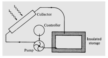
A flat plate collector measuring 2 m × 0.8 m has an overall heat-loss resistance  $R_L = 0.13 \text{ m}^2$ .K/W and a plate efficiency  $\eta_p = 0.85$ . The glass cover has transmittance  $\tau = 0.9$  and the absorptance of the plate is  $\alpha = 0.9$ . Water enters at a temperature  $T_1 = 40$  °C. The ambient temperature
