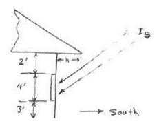
What should the overhang be (h = ?) so that the southfacing window shown in the Figure is shaded at solar noon on June 21<sup>st</sup>. The house is located in Ankara at an elevation of 800 m above sea level.
