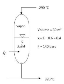
Determine the internal energy of the pressurizer contents before and after the event, in kJ. Ignore heat losses to the ambient.
