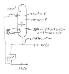
A PWR (Pressurized Water Reactor) has inlet and exit water at 280 °C and 300 °C, respectively. It has a 35 m<sup>3</sup> vapor pressurizer which is normally 30 % full of water at a pressure of 120 bar.
