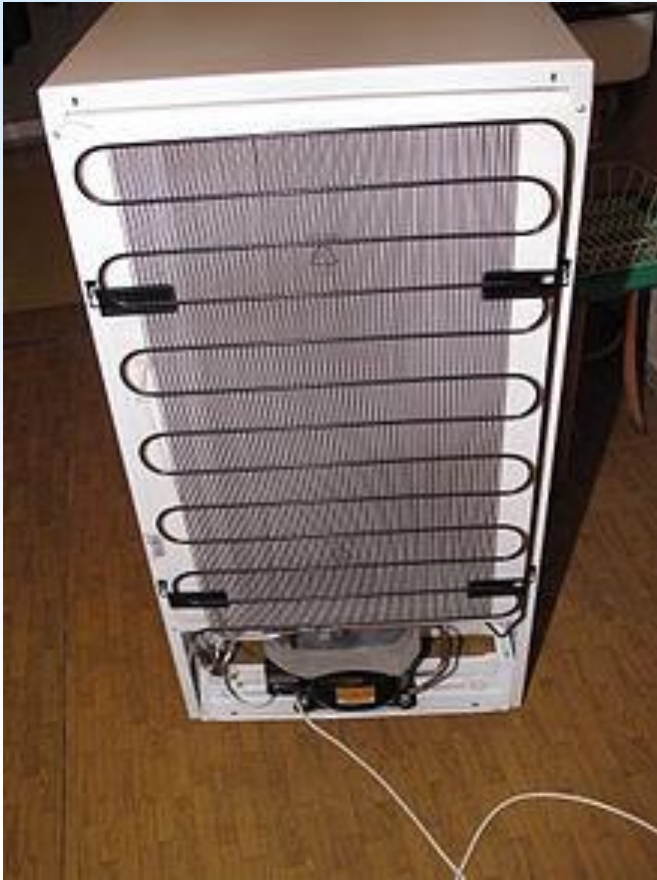
The condensor coil of a refrigerator
