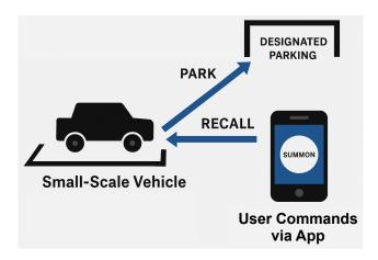
Automated parking and vehicle summon systems represent an important class of advanced driver assistance technologies in the contemporary automotive industry. The aim of this project is to understand and implement the basics of an intelligent vehicle parking and recall system. Students are expected to design and build a small-scale vehicle prototype, including chassis, steering, and drive systems, capable of maneuvering within a compact testbed.
