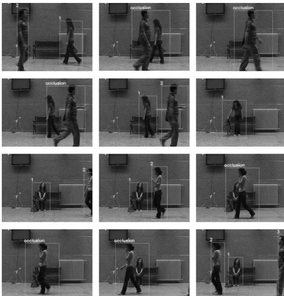
Fig. 7 Example result (handling of multiple occlusions, tracked object is fully occluded) using Set 6
