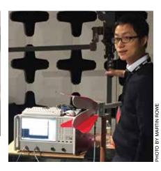
The time domain techniques requires two antennas and an ENA as shown. The technique is included in the draft standard ANSI C63.25 for test site validation and diagnostics.
