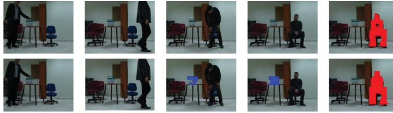
Fig. 10 A handbag is left unattended, when contrast between the background and the handbag is low (floor has low reflectance): (a) Result of the method that does not implement abandoned object detection in thermal data and (b) result of the proposed method.
