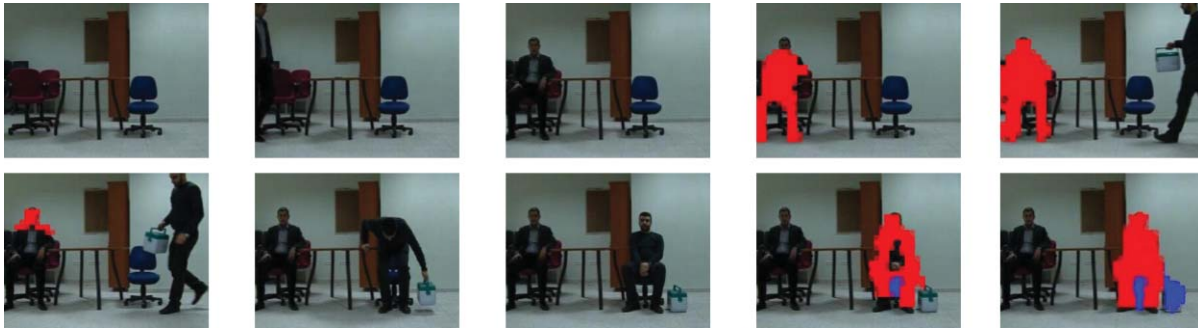
Fig. 6 Result of the proposed method when a handbag is left unattended and the contrast between the background and the handbag is low (low-reflectance floor).
