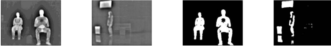
Fig. 3 (a) Thermal images and (b) result of the living-object detection.
